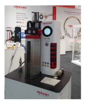
The shrinking process is very gentle in the TubeChiller® using a cooling liquid. During this process, the water level is raised into the tube, and the shrink fit chuck tis cooled circular. If the shrink fit chucks were "showered", the tool would "bend".
